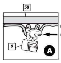
Insert one "arm" of clip into ram as shown. Twist "body" of clip slightly so that second "arm" slides over the top of the first "arm" as shown.
